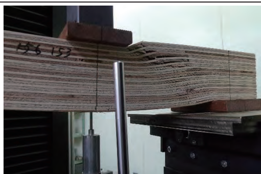
15-3 せん断破壊 1.61N/mm 2
