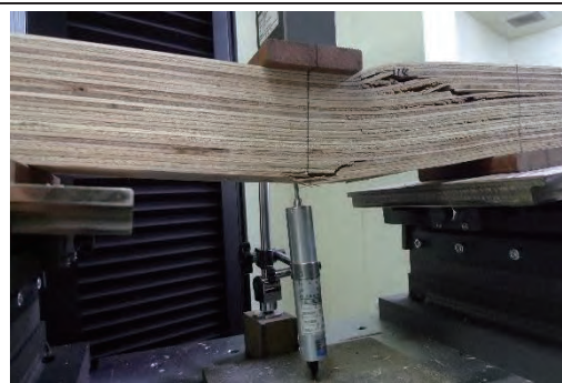
11-4 せん断破壊 1.37N/mm 2
