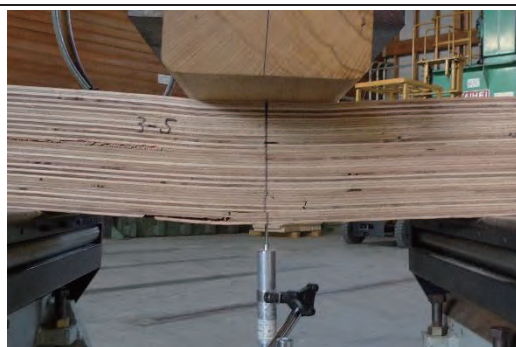
3-5 せん断破壊 1.50N/mm 2
