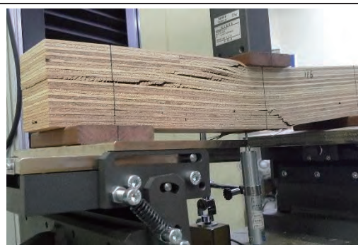
11-6 複合破壊 1.61N/mm 2
