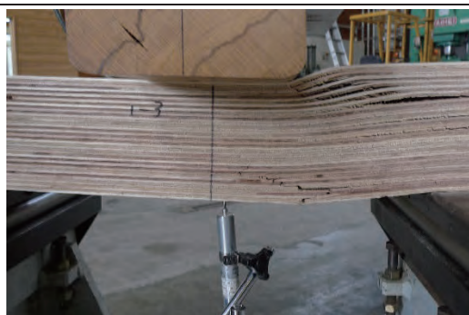
1-3 せん断破壊 1.42N/mm 2
