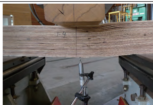
1-4 せん断破壊 1.47N/mm 2
