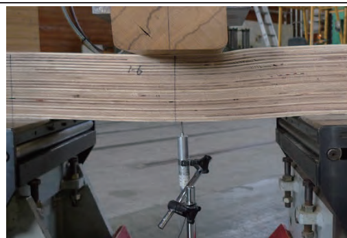
1-6 せん断破壊 1.39N/mm 2
