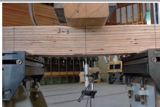
3-3 せん断破壊 1.56N/mm 2
